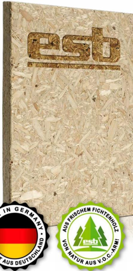
Our specially developed esb board (elka strong board) is a structural wood-based panel according to DIN EN 312:2010. It has excellent technical values and is suitable for use in damp rooms P5. It is ideally suited for structural timber construction. The synthetic resin-bonded chipboard has a single-layer board structure with a combination of fresh sawmill residues.
